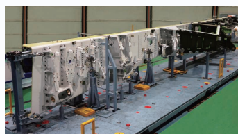
Boeing 787 main wing spar
