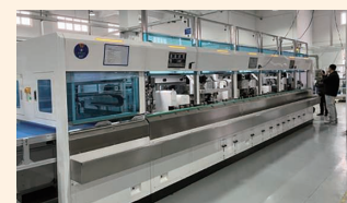
Coaxial cable processor being jointly developed with AST Group (miniFAKRA connectors)
