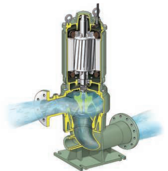
Vertical wet/dry pit type (water-resistant) pump (cross-sectional view)
