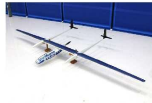
1/5 scale model of high-altitude platform station (HAPS)
