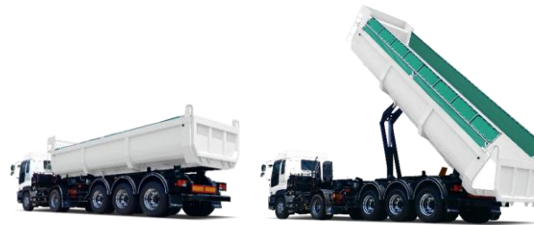
GVW 36-ton dump semi-trailer for transporting soil and gravel
