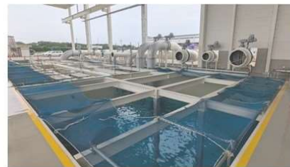
Ono Plant large-scale pump operation inspection equipment (works with pumps up to 1200 mm in diameter)
