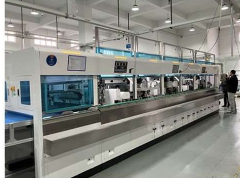
Coaxial cable processor being jointly developed with AST (miniFAKRA connectors)
