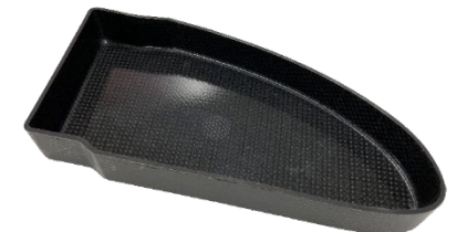
Molded product that imitates aircraft parts made from recycled CFRP
