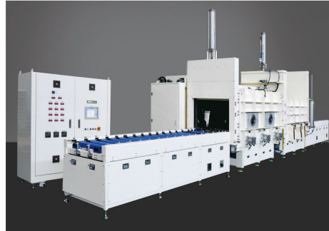
Vacuum driers for secondary batteries for automobiles market
