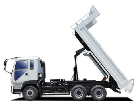
Rear dump body and tipping gear
