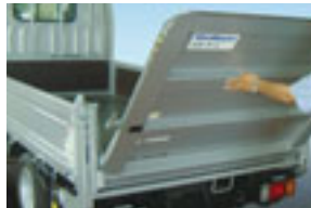
Manually opened/closed platform (support spring equipped)
