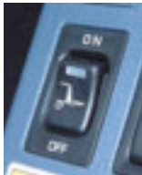
Main switch inside the cabin
