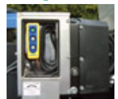
Key-typed main switch (equipped at main remote control box)
