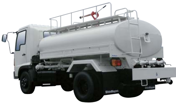
Water Sprinkler with Monitor
