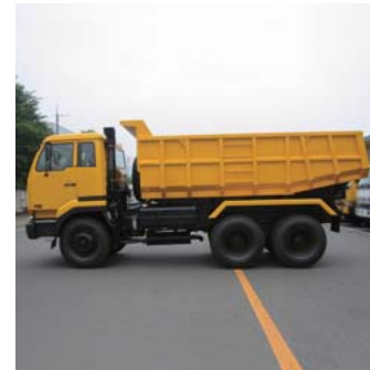
▲ Scoop end type (for rock and heavy material)
