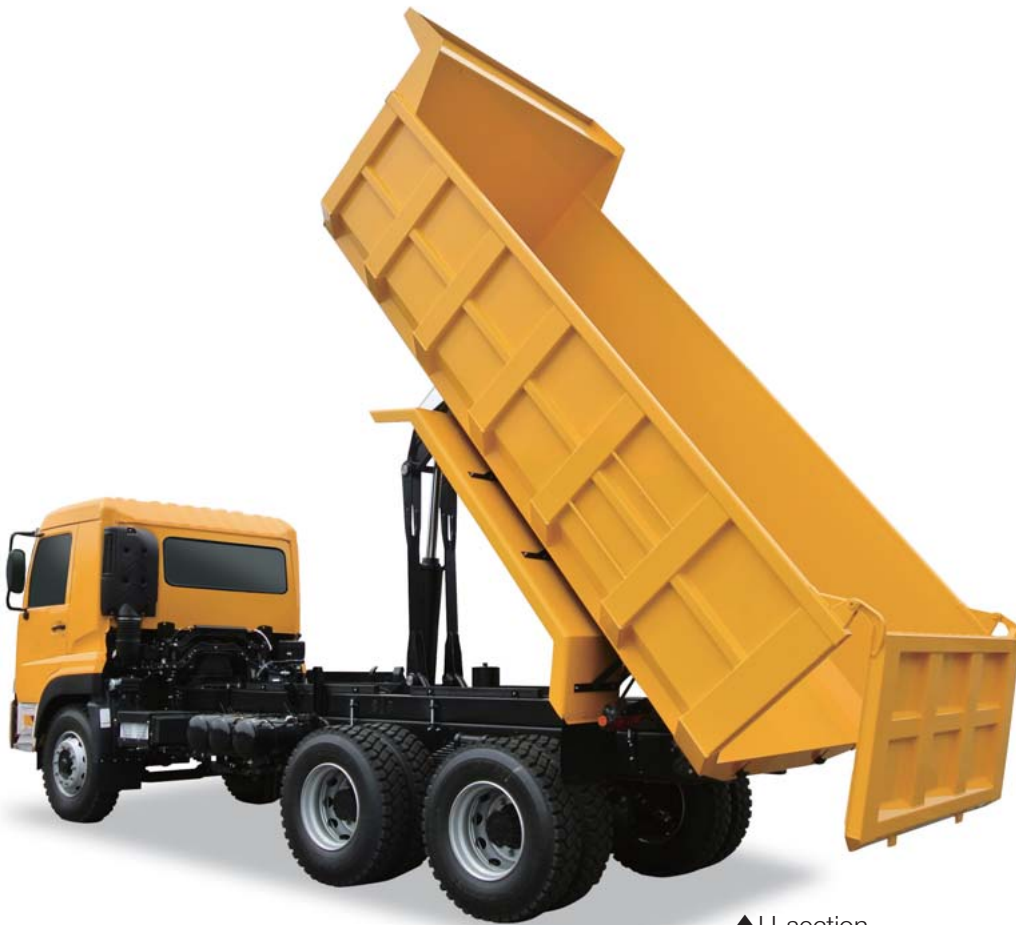
▲U-section drop tailgate type (for sand, soil and gravel)
