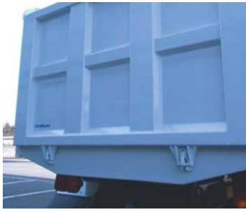
▲ Tailgate opens automatically as the body is raised for dumping.
